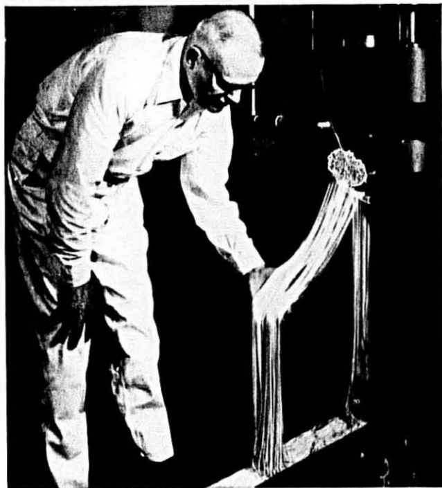
ANOTHER PERFECT TEST RUN. Here, R. C. Benson, Durum Department, checks extrusion from the hydraulic press, a part of the miniature spaghetti plant in operation at Pillsbury's fully-equipped Products Control Laboratory. Capacity of the plant is 20 pounds per hour.
